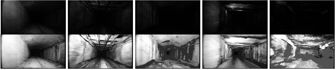
Fig. 1: Top row shows an example of commonly encountered low signal-to-noise ratio imagery from an underground mine captured with a conventional camera. The bottom row shows a histogram-equalized version emphasizing the poor quality and the significant motion blur.
