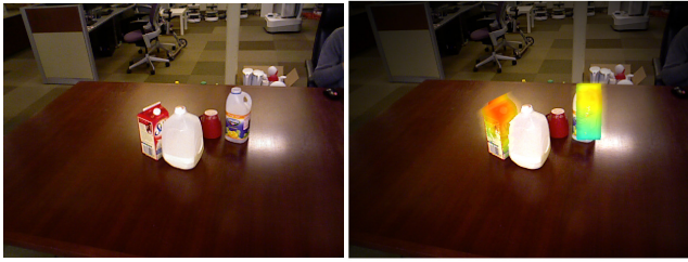
Fig. 5: Example that demonstrates how C-PERCH can be used to obtain pose uncertainty estimates, including multimodal distributions. The object to be localized in this scene ( left ) is the milk carton (for which we have a 3D model) and the other objects are considered as extraneous clutter (no models available). C-PERCH yields two distinct solutions across multiple values of \alpha , which are overlaid on top of the input RGB image ( right ).
