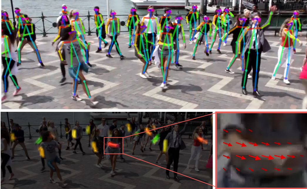
Figure 1. Top: Multi-person pose estimation. Body parts belonging to the same person are linked. Bottom left: Part Affinity Fields (PAFs) corresponding to the limb connecting right elbow and right wrist. The color encodes orientation. Bottom right: A zoomed in view of the predicted PAFs. At each pixel in the field, a 2D vector encodes the position and orientation of the limbs.
