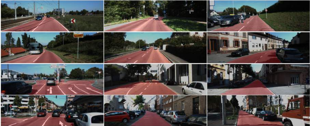
Figure 4.4: Examples of visualization on Kitti road segmentation test set. The road is marked in red.
