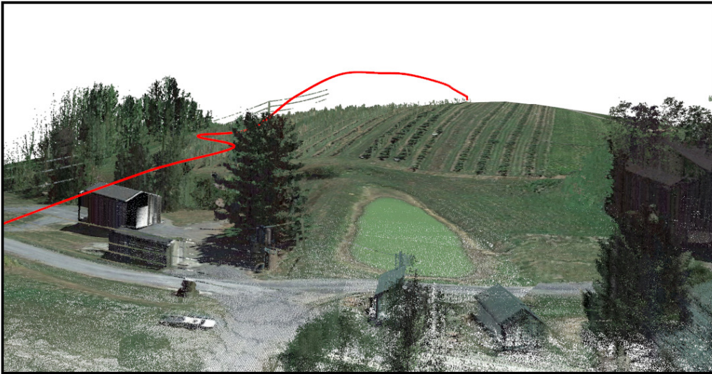
Figure 26: This shows a path planned in a large map which is longer than 500m, whilst avoiding obstacles and adhering to altitude constraints. The point cloud is colorized using aerial imagery, for visualization purposes. (top) The take-off phase of the path is the result of using a funnel constraint. A short vertical section is generated using linear interpolation and the smooth, curved transition comes from using a large-radius funnel-shaped constraint. (bottom) The path goes around obstacles that exist in the static map, like the big tree. An altitude constraint of 15–17m makes the shape of the path match the ground terrain below it.
