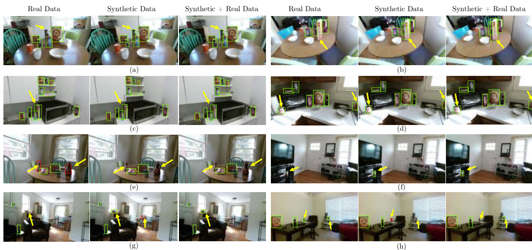
Figure 4.8: We show qualitative detection results and mark true positives in green, false positives in red and arrows to highlight regions. The top two rows are from the GMU Kitchen Scenes 13 and the bottom two rows from the Active Vision Dataset 1 . (a), (b): Model trained on real data misses objects which are heavily occluded (a) or stops detecting objects as viewpoint changes from a to b. (c), (d): Model trained on synthetic data detects occluded and truncated objects. (e): Combining synthetic data removes false positives due to training only on real data. (g), (h): Combining real data removes false positives due to training only on synthetic data. (f), (g): Viewpoint changes cause false negatives. (Best viewed electronically)
