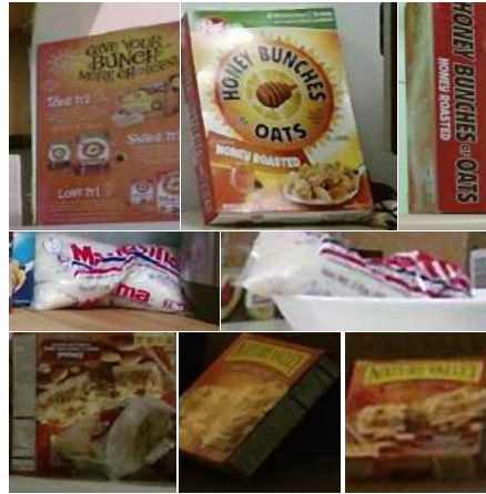
Figure 4.6: Missed detections on the Active Vision Dataset 1 for a model trained on the hand-annotated GMU Dataset 13 . The model consistently fails to detect certain viewpoints as the training data has poor viewpoint coverage and has biases different from the test set. Each row shows a single instance.
