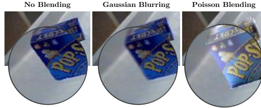
Figure 4.4: Different blending modes used while generating datasets. These modes help the model in ignoring artifacts arising from pasting objects on background scenes. More details in Section 4.4.2
