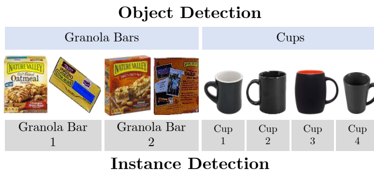
Figure 1.1: Object vs Instance Detection. Instance detection involves fine-grained recognition within the same ‘object category’. In this example, instance recognition must distinguish amongst 6 classes: 2 types of granola bars and 4 types of coffee cups. Object detection would distinguish only amongst 2 classes: coffee cups and granola bars. Instance detection must model minute differences between instances of the same generic object category.
