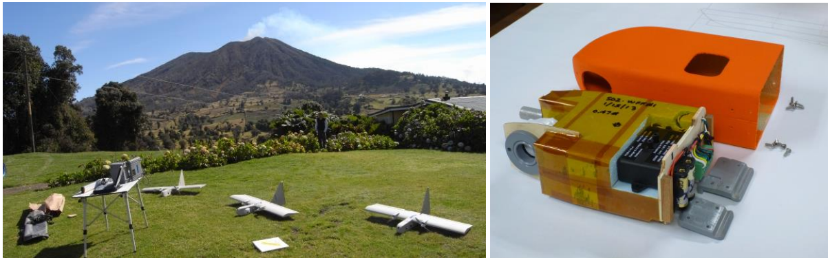
Figure 4. NASA Ames Dragon Eye UAS deployed at the Turrialba Volcano in Costa Rica in 2013 (left), and the SO 2 sensor payload developed at NASA Wallops Flight Facility (right).
