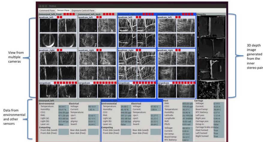
Fig. 4: User interface showing the camera view. The top section streams camera data from the different cameras along with a 3d depth image generated using the top inner stereo pair cameras. The bottom section shows the data streaming from the environmental and other sensors.
