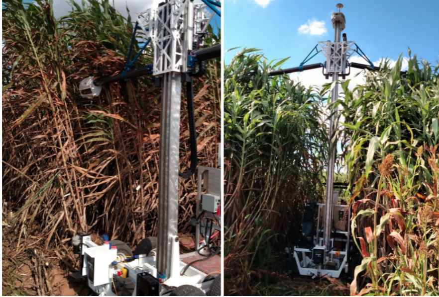
Fig. 1: High-throughput Phenotyping robot in a sorghum field in Weslaco, Texas. Sorghum grows 6 meters tall in 4 months.
