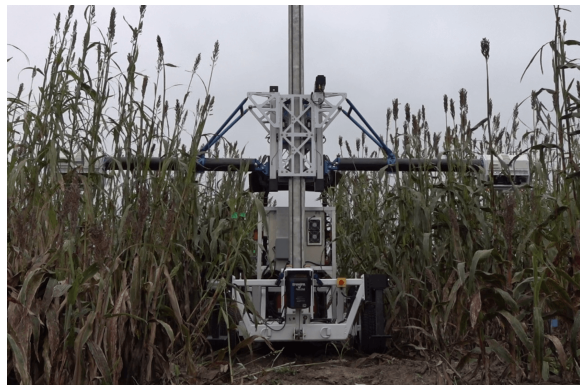
Fig. 1. High throughput phenotyping platform deployed in a sorghum field outdoors. The platform has two arms on either side that extend outwards into crop rows and scan plants vertically at a resolution of 10 cm. Each arm is fitted with two multi-camera sensorpods facing front and back.
