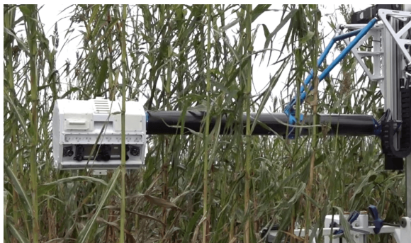
Fig. 7. A closeup of the multi-camera sensor pod deployed on the robotic platform. The sensor pod contains eight forward facing and two additional cameras verged on either ends at an angle of 30^\circ . The sensor pod is connected to a robotic arm and can collect images at multiple plant heights.
