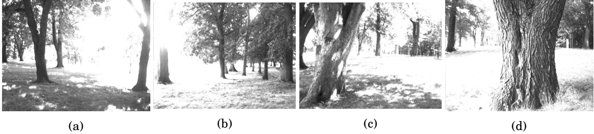
Figure 3.4: Examples of images that failed during flight. Failures were resolved by (a) rotating left, (b) rotating right, (c) translating left, and (d) translating right. Intuitive causes of failure include direct glare from sunlight (c,d), strong shadows (b, d), open area (b,c), large obstacles preventing adequate parallax (a), and overexposure (a,c,b). Our algorithm used thousands of images like these to learn which trajectories are most likely to recover from perception failures.
