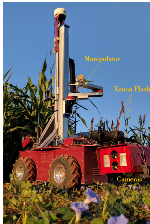
Figure 3.2: A custom side-facing stereo camera for phenotyping.
