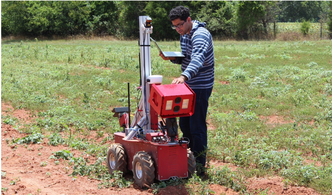
Figure 6.1: Stereo camera mounted on “The Robotanist” [45].
