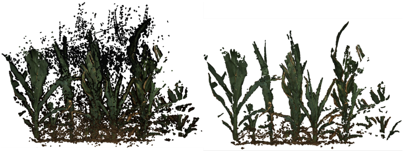
Figure 6.2: Left: point cloud before filtering; Right: point cloud after removal of dark pixels and statistical outliers.
