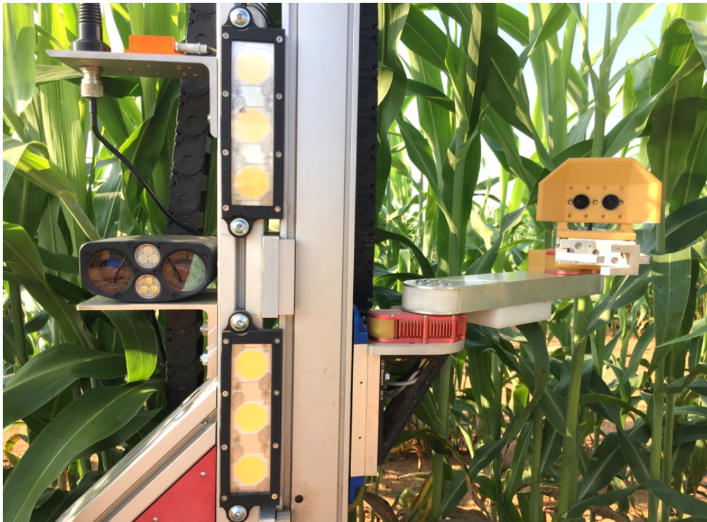
Figure 7.1: Left: The Multisense S7 is mounted horizontally to the robot mast; Center: Two custom flash boards are mounted vertically on the mast between the Multisense S7 and the first joint of the manipulator; Right: The DUO3D camera is still mounted to the manipulator, but it is unused
