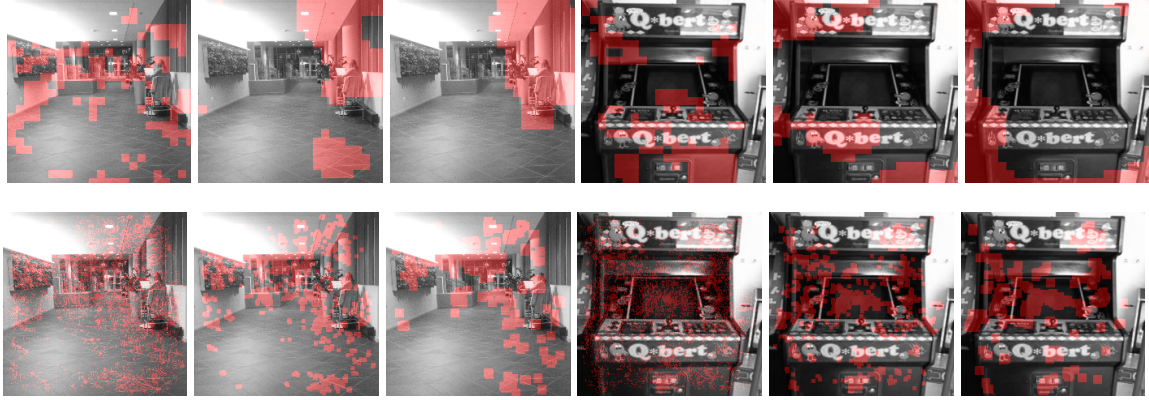
Figure 3.4: The image masks for the (top) occ importance function and (bottom) grad importance function generated with the parameters \rho=25\% and with dilation = \{0, 2, 5\} respectively for one image from the Building-Floor dataset (left three images) and one image from the Places365 dataset belonging to the class amusement station (right three images).
