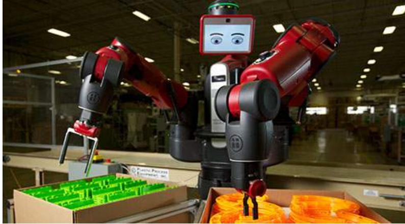
Figure 2: Rethink Robotics ® Baxter compliant robot working on an assembly line [7]
