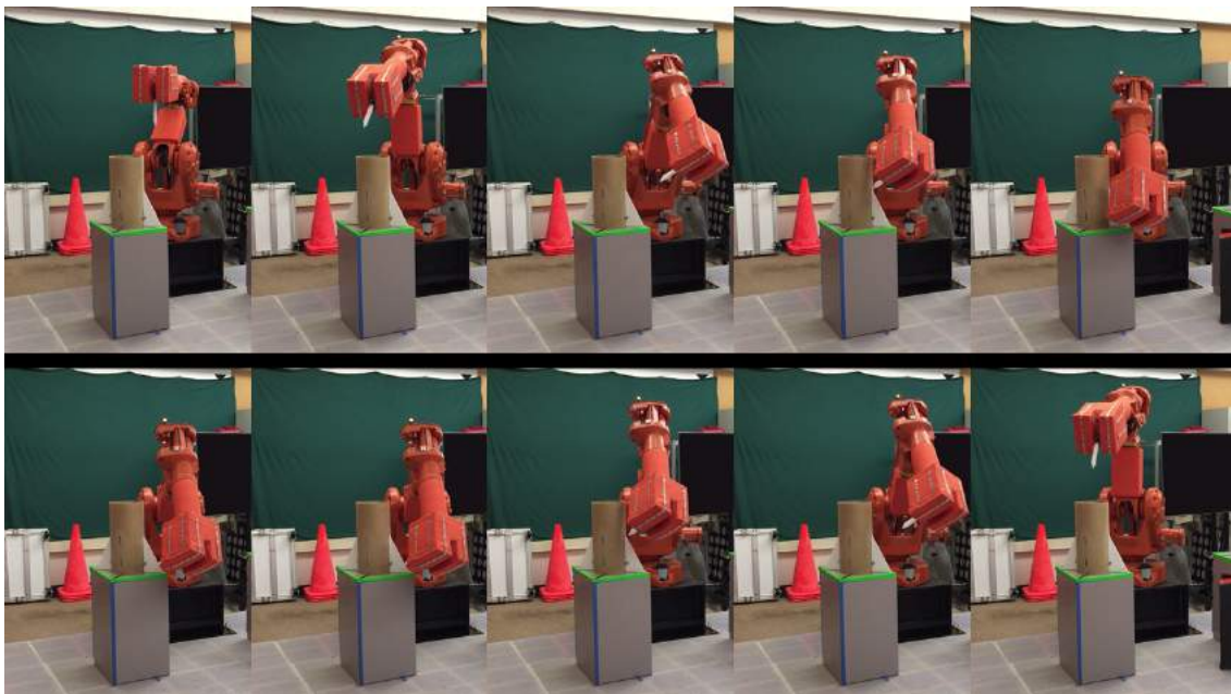
Figure 17: Robot completing its simulated weld: runs the foam welding “tip” along the fin seam at reduced speed
