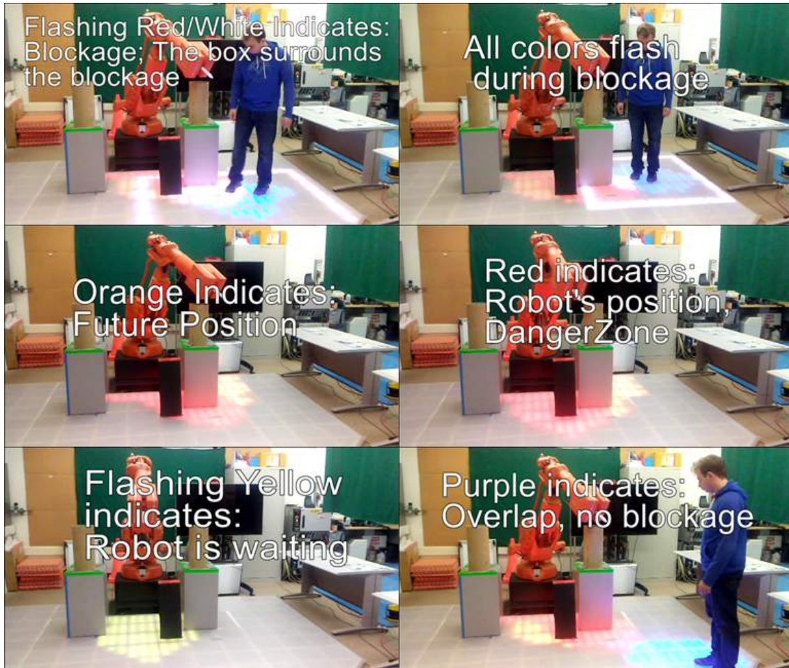
Figure 18: Floor display video tutorial. Describes the different states and coupled information: blocked state along with the blockage localizing box and overlaps, running state with the robot danger zone and future position, and the passive waiting state.
