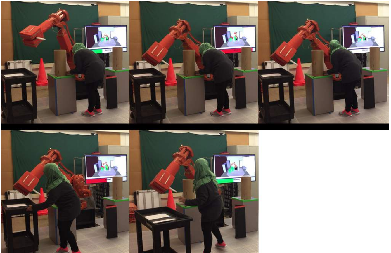
Figure 30: Responsive Reaction (shown with the simulation): robot and worker are completing tasks in parallel. Robot becomes blocked. Worker observes the feedback. Worker takes immediate or near immediate action to correct the blockage. Robot and worker both resume tasks. Feedback is observed, and corrective action is taken.
