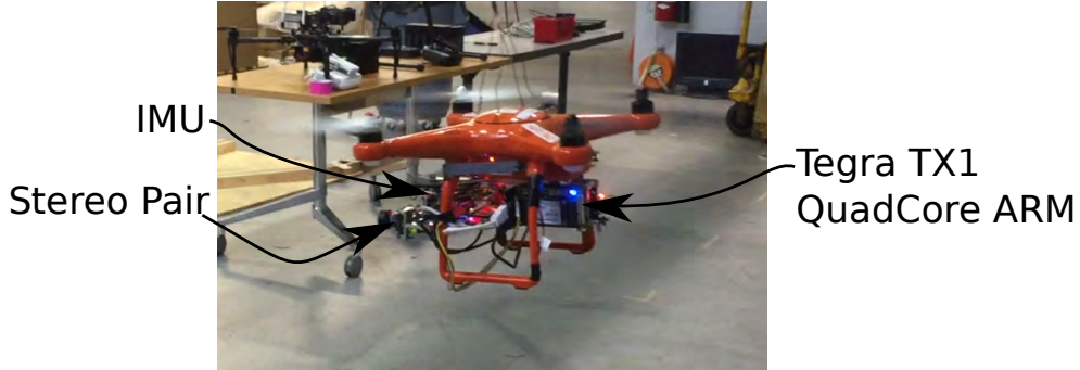
Figure 5.19: A smaller quadrotor platform used for experiments: equipped with stereo camera sensor suite and onboard ARM computer
