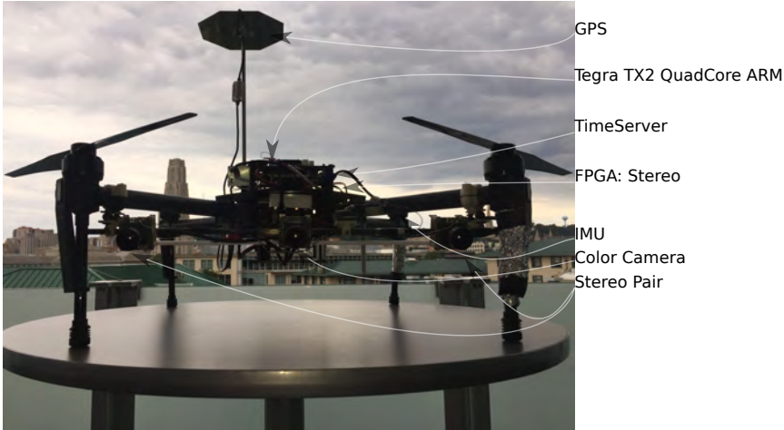
Figure 5.12: Quadrotor platform used for 10m/s runs: equipped with stereo camera sensor suite and only one onboard ARM computer. This helped in significant weight reduction of about 33%, from 1.2Kg to 0.8Kg.
