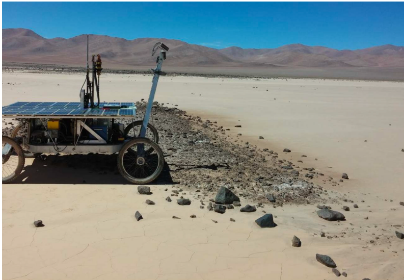
Figure 2.1: Example of the CMU rover Zoë navigating autonomously in the Atacama Desert, Chile. Zoë is collecting data with its spectrometer from a location of interest for the science team.
