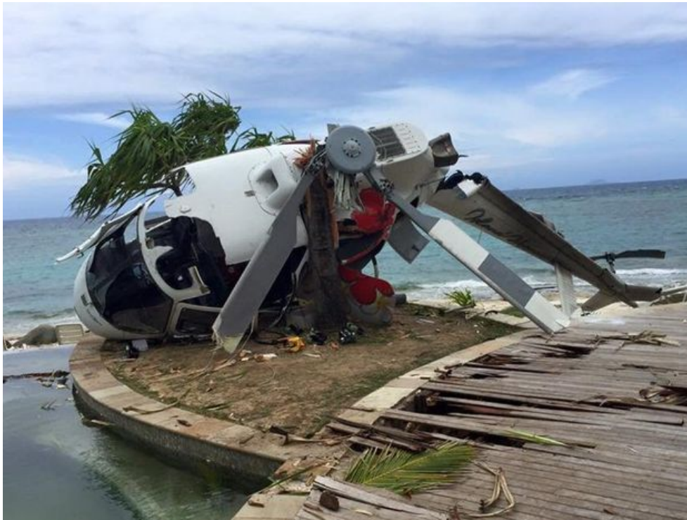
Figure 1.2: A helicopter crash in Fiji. A strong gust of wind destabilized it as it attempted to land.
