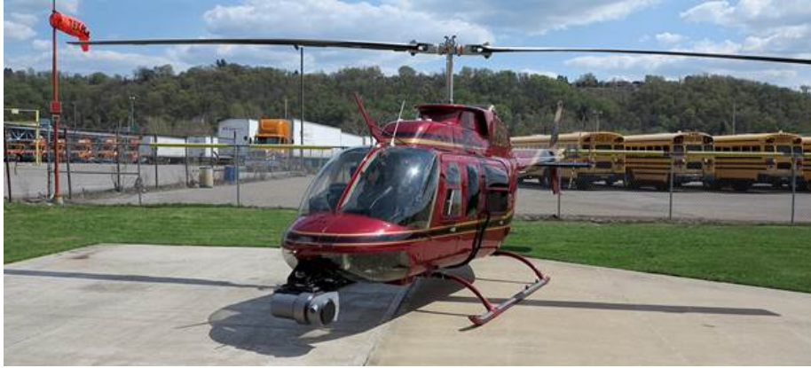
Figure 6.4: Our autonomous helicopter test platform. The laser sensor is visible at the nose of the vehicle.
