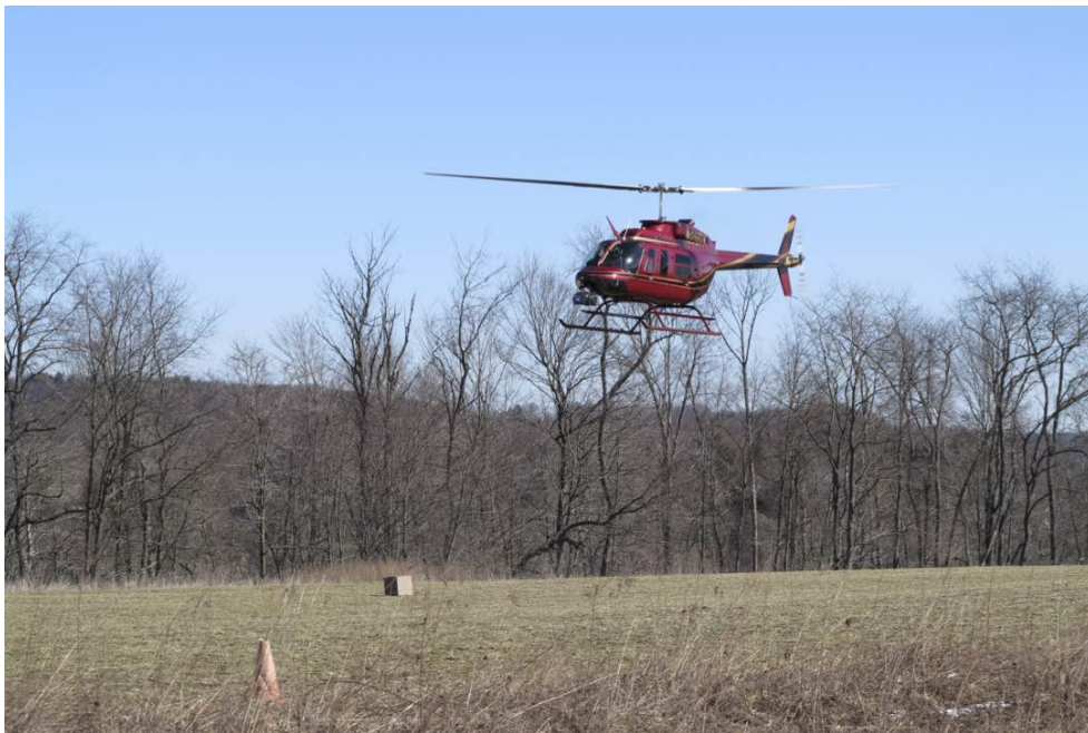
Figure 1.1: A modified Bell 206 serves as one of our autonomous helicopter test platforms.
