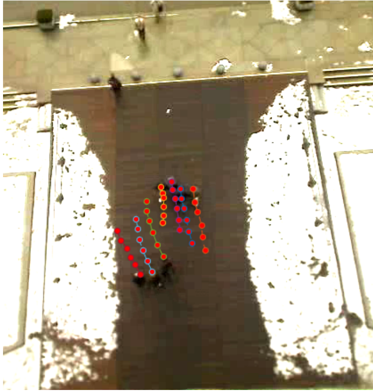
Figure 4.4: Example prediction by our model. For each pedestrian, we predict his future locations (which are plotted) for the next 5 time-steps. The bottom set of pedestrians are progressing towards a goal at the top centre of the image, but they go around the other set of pedestrians making way for them cooperatively.
