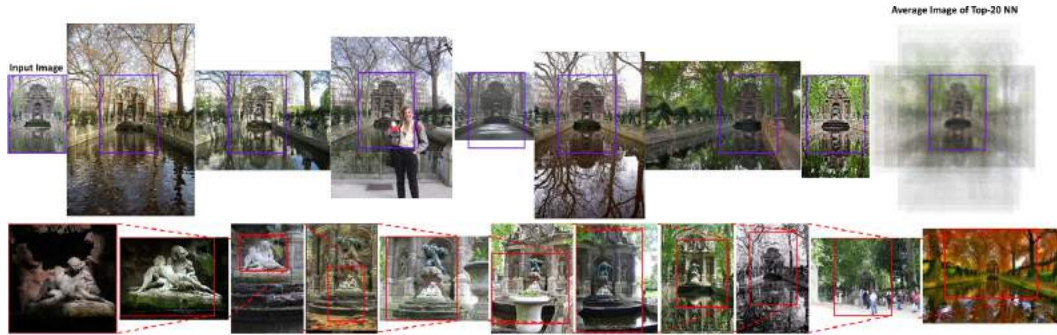
Figure 7.15 – Visual Scene Exploration. (Top): Given an input image, we show the top matches, aligned by the retrieved sub-window. The last image shows the average of top 20 matches. (Bottom): A visualization of the memex-graph tour through the photos of the Medici Fountain.
