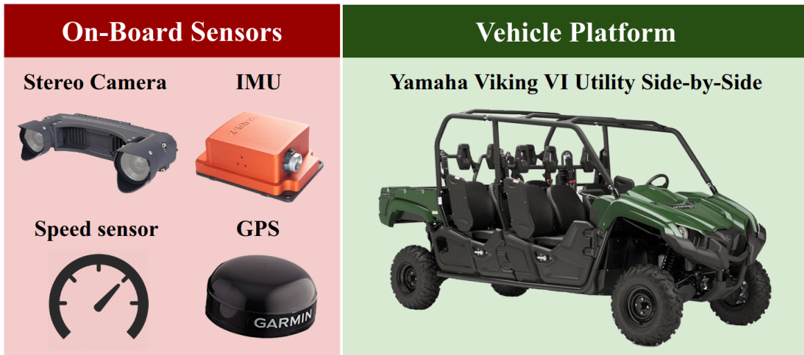
Figure 2.1: The testing vehicle and on-board sensors.
