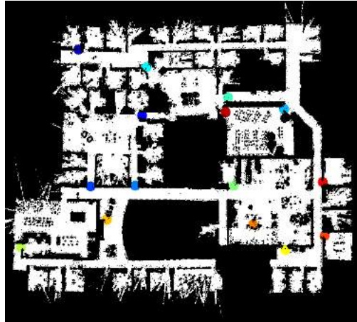
FIGURE 7.6: The 2D grid map used for synthetic benchmarking experiments. The 15 colored circles represent regions (and consequently edges) in the grid that exist with some probability, and are also expensive to evaluate.
