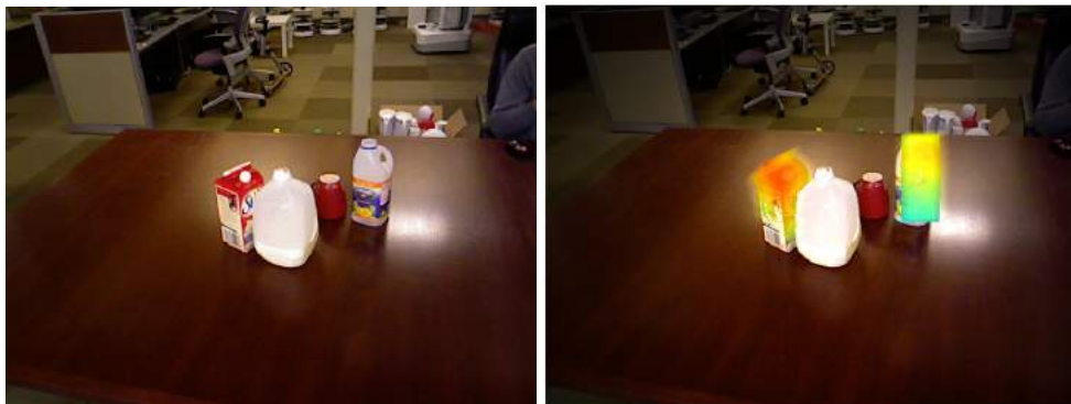
FIGURE 4.3: Example that demonstrates how C-PERCH can be used to obtain pose uncertainty estimates, including multimodal distributions. The object to be localized in this scene ( left ) is the milk carton (for which we have a 3D model) and the other objects are considered as extraneous clutter (no models available). C-PERCH yields two distinct solutions across multiple values of \alpha , which are overlaid on top of the input RGB image ( right ).
