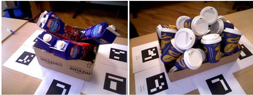
FIGURE 9.2: Examples from the dataset in (Doumanoglou et al., 2016) where consideration of physics constraints is required to reliably estimate 6 DoF poses of all objects in the scene.
