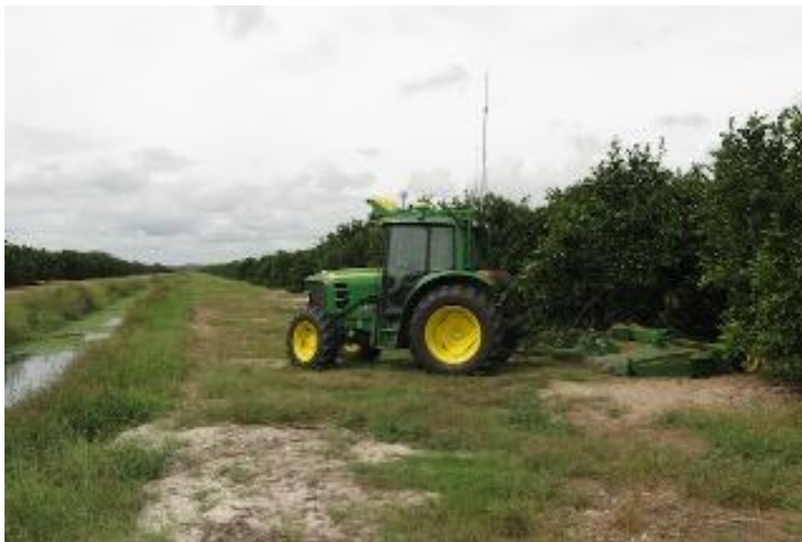
Figure 5: Autonomous Orchard Tractor turning at the end of the row.
