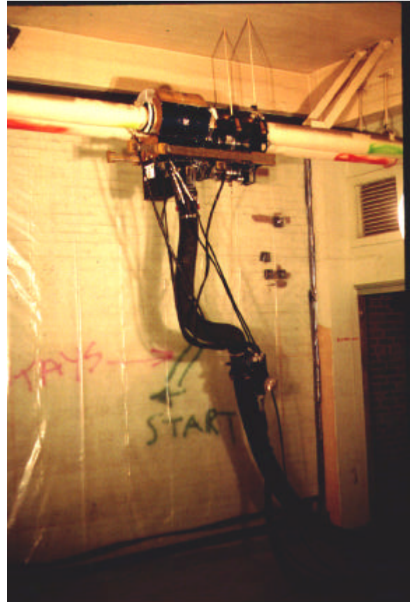
Figure 21: BOA installed on pipe in Pentagon
