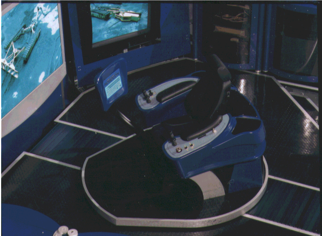
Figure 6: RoboCon Operator Platform: Chair, Panels and Touch-screen
