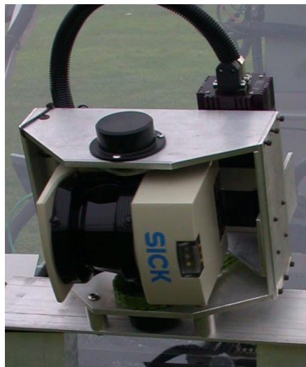
Figure 5 Sweeping laser scanner consists of a commercial single axis scanner that is panned in a fan like motion to generate an elevation map of the terrain ahead of the vehicle.
