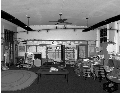
Figure 7. A schoolhouse which we are using as a case study for modeling. Top: The combined point cloud from all of the scans. Bottom: A portion of the reflectance image from one scan, showing the degree of clutter in the natural environment.
