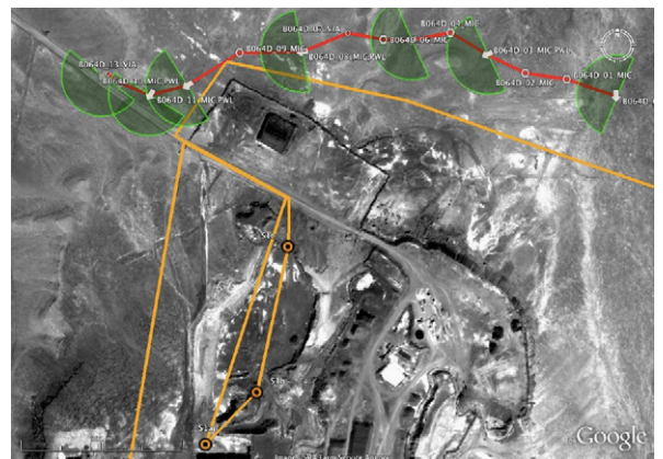
Fig. 9. Trafficability of N1 (orange) is a concern north of S1c. Recon (red) addresses this via panoramic images (field-of-view is shown in green). (For interpretation of the references to colour in this figure legend, the reader is referred to the web version of this article.)
