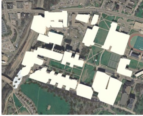
Figure 4.1: The virtual campus environment of Carnegie Mellon University, Pittsburgh, PA that is used in the simulation experiments. Buildings that were added to the digital elevation model are shown in white. A hemispherical 200m range 3D range sensor is simulated to update the environment map held by the robot.
