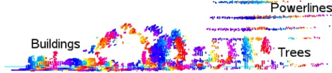
Figure 3.18: A scene generated from a series of static scans of the environment with buildings, trees and powerlines. The powerlines are visible at 170m.
