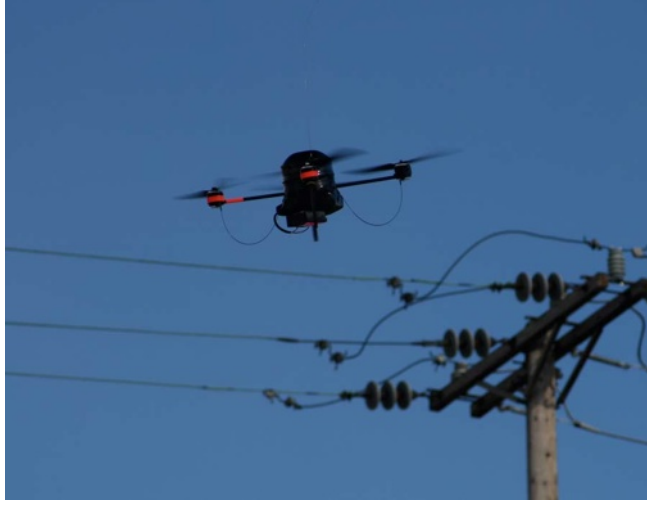
Figure 4.2: The autonomous quad-rotor aerial vehicle used for testing. Here, the vehicle is close to a typical pole and wire obstacle in the environment. The system is equipped with a computer, a GPS, an inertial measurement unit, and a ladar scanner to sense the environment. The size of the vehicle with rotors is less than one meter.
