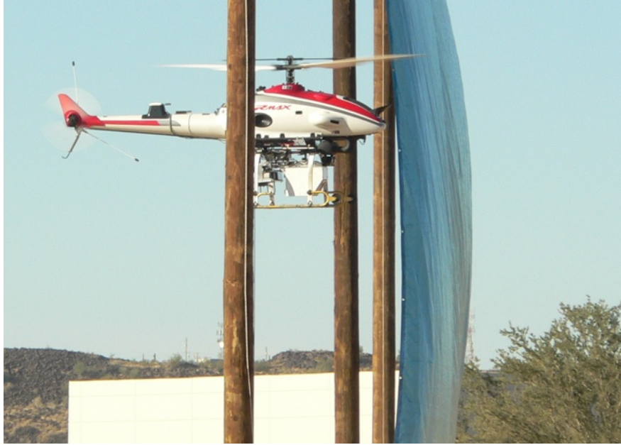
Figure 3.1: The helicopter platform we used to test collision avoidance flying autonomously between two poles 10 m apart. The rotor span of this helicopter is 3.4 m
