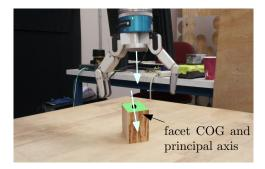
Figure 6: The Barrett hand in a cup pre-shape is positioned above the center of gravity of the facet (marked in green), and alligned with respect to the facet's prinicpal axis.
