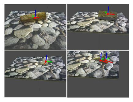
Figure 5: Experimental evaluation of action generation based on the detected facets. Each column corresponds to a single object configuration of the 4 objects in Figure 4. The 3D view shows the object. The center of gravity is marked by a red sphere. The object's axes are color coded: principal axis (red), secondary axis (green), and trinary axis (blue). In all cases the position of the center of gravity and orientation of the axes correspond well with the object.
