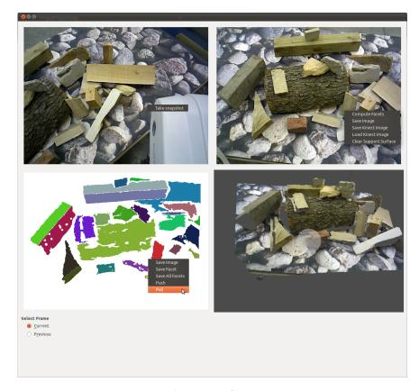
Figure 8: The Graphical User Interface. **Top left:** Live video. The operator can choose when to take a snapshot of the scene using a context menu. **Top right:** The captured snapshot. It is updated when a new snapshot is requested. The interface can show either the current or previous snapshot (radio button on bottom left). **Bottom left:** The computed facets. The operator can choose from a list of available action by right-clicking on each facet. **Bottom right:** A live 3D display.
