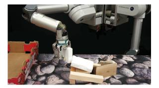
Figure 1: Andy (DARPA's ARM-S platform) manipulating a clutter of natural objects taken from a construction site.
