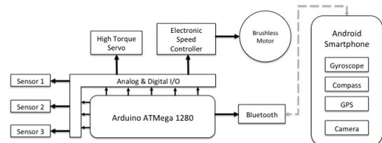
Figure 2: Hardware functional diagram.
