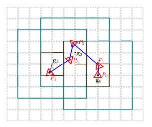
Fig. 2. In this figure the global position of the TSDF (denoted by  $\mathbf{g}_i$ ) is updated twice over the course of five frames. The continuous pose of the camera  $P_i$  is shown for each of the five frames. The current TSDF virtual window in global space is shown in teal, the current movement boundary is shown in dark brown and the underlying voxel grid quantization is shown in light dashed lines. This simplified example has b=1 and  $v_s=6$ .
