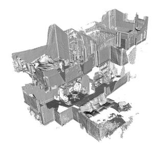
Fig. 1. Real-time 6DOF extended scale map reconstruction of a dataset captured using a handheld Kinect traversing multiple rooms over two floors of an apartment. (see Section V-B)
