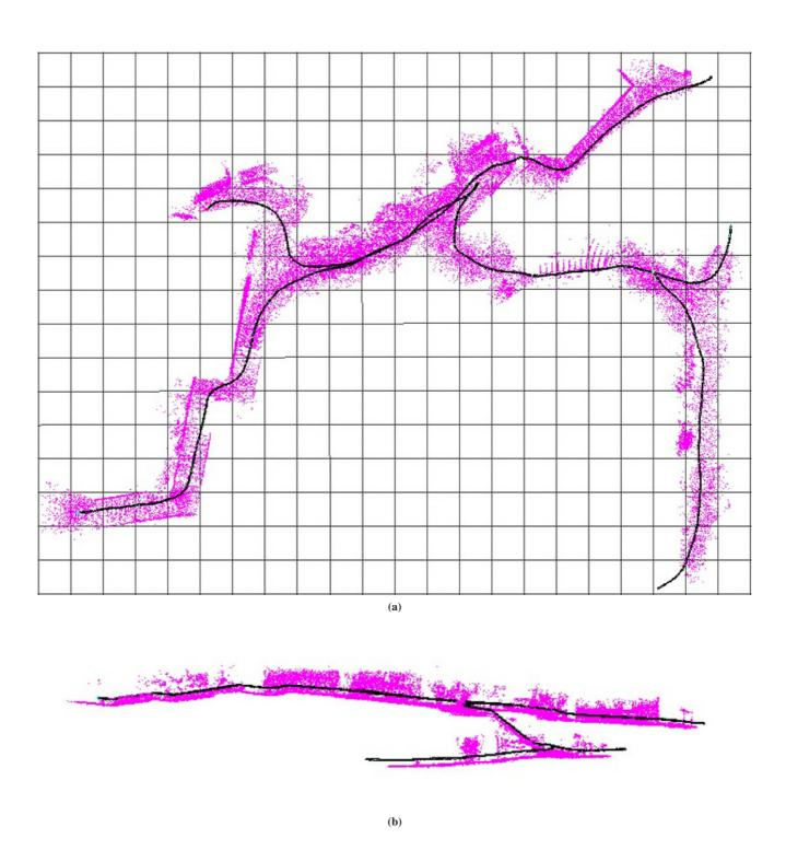
**Figure 13:** Multi-session results for outdoor datasets from Experiment 3 including 3 sessions. (a) shows a plan view where the grid is at a scale of 5m. (b) shows an orthographic side view where the full 3D structure is apparent, in particular the stairs. See Section 4.2 for further details.
