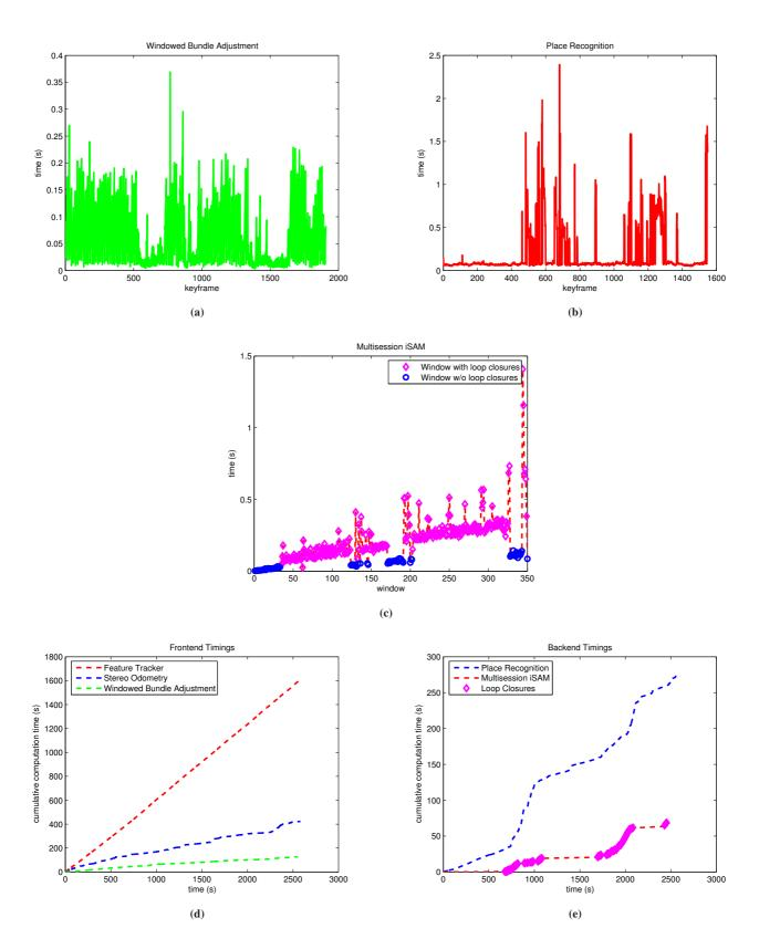
**Figure 10:** Timings for Experiment 2: multi-session indoor sequences. (a) and (b) show the processing times per keyframe for windowed bundle adjustment and place recognition, respectively. (c) shows the processing time for multisession iSAM for each window, distinguishing between windows with and without loop closures. (d) and (e) show the cumulative processing time for the individual modules of the frontend and backend, respectively.
