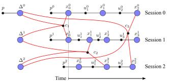
(d) The relative pose graph formulation generalizes to more than two sessions, and does not require the pose graphs to be synchronized or even to start at the same time or location. This example shows three encounters between three sessions.
