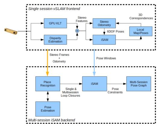
Figure 1: Internal architecture of windowed and multi-session visual SLAM (vSLAM) processes.
