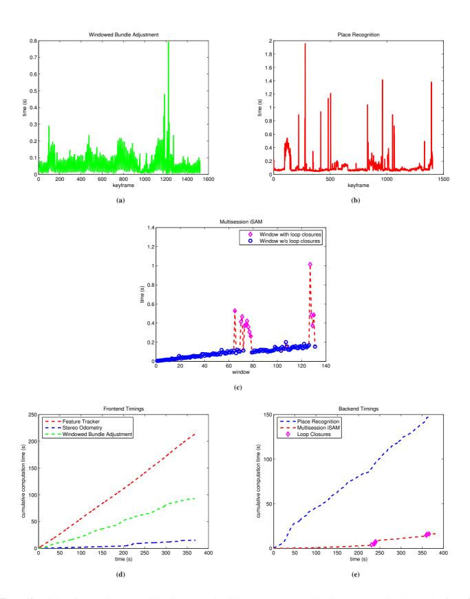
**Figure 12:** Timings for Experiment 3: multi-session outdoor handheld sequences. (a) and (b) show the processing times per keyframe for windowed bundle adjustment and place recognition, respectively. (c) shows the processing time for multisession iSAM for each window, distinguishing between windows with and without loop closures. (d) and (e) show the cumulative processing time for the individual modules of the frontend and backend, respectively
