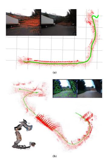
**Figure 5:** Single session visual SLAM processing including full 6-DOF motion.
