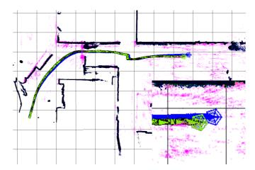
**Figure 6:** Comparison of drift in single session visual SLAM against 2D LiDAR scan matcher over a 20m trajectory. Grid scale is 2m. (For interpretation of the references to colour in the text, the reader is referred to the web version of this article.)
