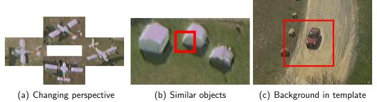
Figure 4.3: Examples showing two cases, (a) and (c), for which non-spatial tracking dominates, and another, (b), for which a spatial template is more appropriate.
