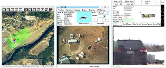
Figure 4.2: Screenshots of the overhead map view, UAV, and UGV control window components of the common operator interface for unified collaborative control.
