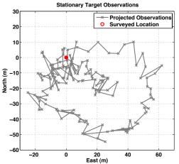
Figure 4.6: Observations of a stationary target over one orbit, exhibiting large, time-varying bias.
