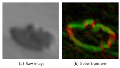
Figure A.2: The image patch template that is tracked in the video stream.
