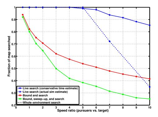
Figure 6.26: Fraction of the entire surrounding environment eventually searched vs. searcher-to-target speed ratio when performing a guaranteed search for a bounded-speed target in a  $3 \text{km} \times 2 \text{km}$  road network with 40% edge density and block (edge) lengths of 200m (roughly, urban). The number of agents available to each strategy corresponds to the matching datapoint in Figure 6.20, that is, the minimum team size providing a capture solution is used in each instance.
