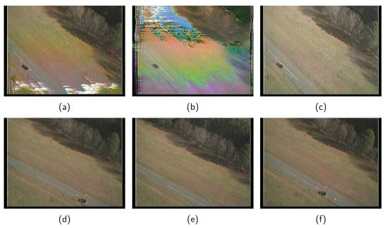
Figure A.6: Different types of tracking recovery. The top row shows the tracking recovery after a period of communications corruption. The bottom row shows the tracking recovery after the target leaves the field of view. This figure is duplicated for viewing convenience from Figure 4.4.
