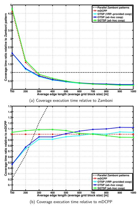
Figure 5.19: Coverage execution time comparison between Zamboni patterns and the greedy mDCPP competitor, orbit OTSP (OTSP) using both a VRP solver and an adhoc spatial split of the environment into independent TSPs, and sweeping generalized TSP (SGTSP) algorithms for 3 UAVs running in parallel.
