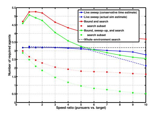
Figure 6.29: Required team size vs. searcher-to-target speed ratio used to perform a guaranteed search for a bounded-speed target in a  $3 \text{km} \times 2 \text{km}$  road network with 40% edge density and block (edge) lengths of 200m (roughly, urban). The number of agents available to each strategy is fixed at 10, and more than strictly necessary may be used to reduce search time (area). Where obscured by legend, traces are roughly linear.
