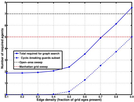
Figure 6.10: Comparison of required team size to perform a guaranteed search of a possibly cycle-containing road network of fixed  $3 \text{km} \times 2 \text{km}$  size and 450 m edge lengths but varying edge density, from 10% to 90% of all edges in the underlying grid present. For reference, note that environments with these parameters and edge density 0.5 is considered canonically suburban in this document.
