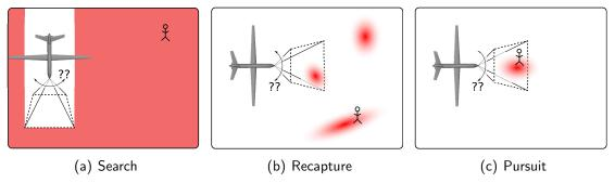
Figure 2.1: Intuitive depictions of pursuit, recapture, and search, along with the need to steer the path of the observer. Red shading indicates the relative probability of target presence, and the trapezoidal region leading the UAV indicates the region visible to it (formalized in Section 2.7).
