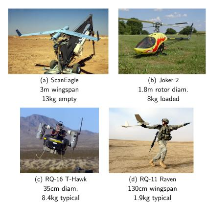
Figure 1.3: Examples of small field-reconnaissance UAVs considered primarily in this thesis, such as the Insitu ScanEagle catapult-launched and hook-retrieved tactical surveillance UAV, (a) the Maxi-Joker 2 camera-transport helicopter, (b) the Honeywell RQ-16 T-Hawk vertical takeoff and landing ducted-fan UAV, (c) and the hand-launched AeroVironment Raven local reconnaissance UAV. (d)
