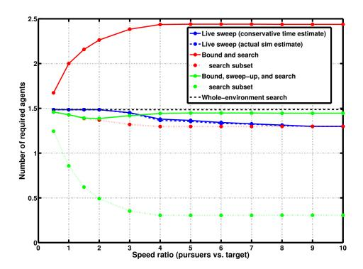
Figure 6.31: Required team size vs. searcher-to-target speed ratio used to perform a guaranteed search for a bounded-speed target in a  $3 \text{km} \times 2 \text{km}$  road network with 40% edge density and block (edge) lengths of 700m (roughly, rural). The number of agents available to each strategy is fixed at 10, and more than strictly necessary may be used to reduce search time (area).
