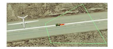
Figure 4.17: Visualization example from simulation showing a UAV pursuing a Jeep. The green trapezoid is the ground region visible to the camera. The orange dot indicates the geolocation filter's best estimate of the target's position at the center of the red smear denoting the surrounding uncertainty distribution.
