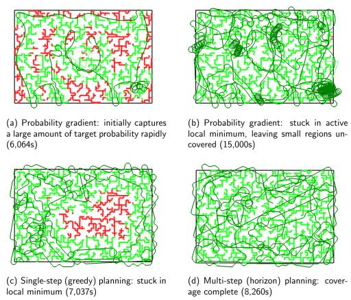
Figure 5.16: Sample execution results for three traditional environment-aware algorithms attempting to maximize short-term probability of detection in an urban-density environment. Of these, only multi-step planning (requiring 3.8s per planning step, which is infeasible for realtime execution) completes coverage.
