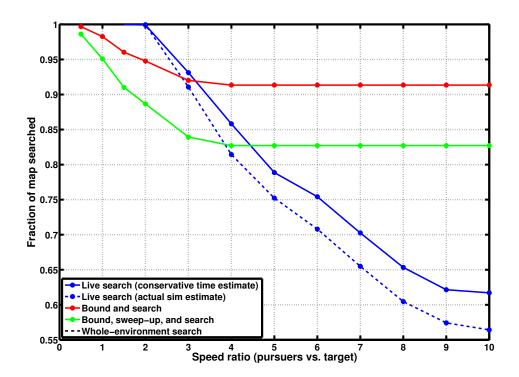
Figure 6.28: Fraction of the entire surrounding environment eventually searched vs. searcher-to-target speed ratio when performing a guaranteed search for a bounded-speed target in a  $3 \,\mathrm{km} \times 2 \,\mathrm{km}$  road network with 40% edge density and block (edge) lengths of 700m (roughly, rural). The number of agents available to each strategy corresponds to the matching datapoint in Figure 6.22, that is, the minimum team size providing a capture solution is used in each instance.
