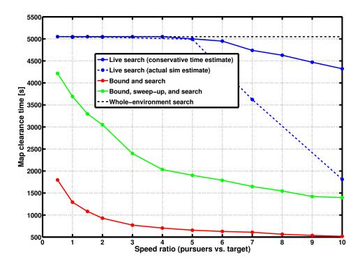
Figure 6.23: Comparison of mission duration with increasing searcher-to-target speed ratio to perform a guaranteed search for a bounded-speed target in a  $3 \text{km} \times 2 \text{km}$  road network with 40% edge density and block (edge) lengths of 200m (roughly, urban). The number of agents available to each strategy corresponds to the matching datapoint in Figure 6.20, that is, the minimum team size providing a capture solution is used in each instance.
