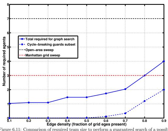
Figure 6.11: Comparison of required team size to perform a guaranteed search of a possibly cycle-containing road network of fixed  $3 \text{km} \times 2 \text{km}$  size and 700 m edge lengths but varying edge density, from 10% to 90% of all edges in the underlying grid present. For reference, note that environments with these parameters and edge density 0.5 is considered canonically rural in this document.
