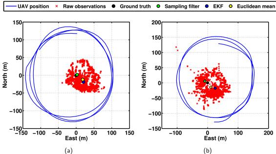
(a) (b) Figure 4.11: Plot of geolocation results from two test flights, under both (a) low to moderate wind and (b) high-wind conditions. The evidence-grid error-sampling filter outperforms an EKF and a naive Cartesian mean in both cases.
