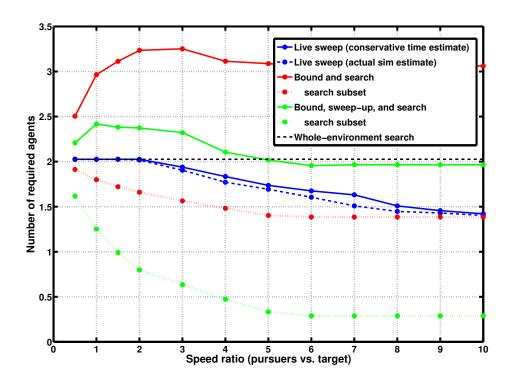
Figure 6.30: Required team size vs. searcher-to-target speed ratio used to perform a guaranteed search for a bounded-speed target in a  $3 \text{km} \times 2 \text{km}$  road network with 40% edge density and block (edge) lengths of 450 m (roughly, suburban). The number of agents available to each strategy is fixed at 10, and more than strictly necessary may be used to reduce search time (area). Where obscured by legend, traces are roughly linear.
