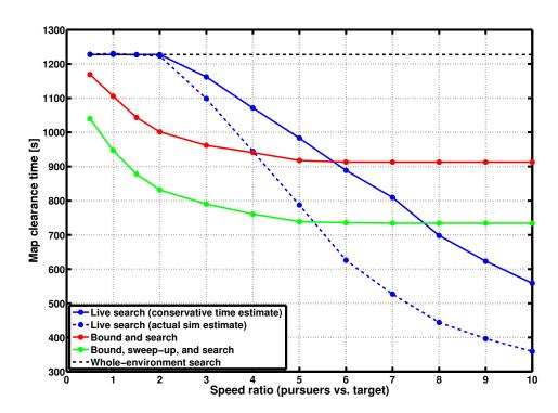
Figure 6.24: Comparison of mission duration with increasing searcher-to-target speed ratio to perform a guaranteed search for a bounded-speed target in a  $3 \text{km} \times 2 \text{km}$  road network with 40% edge density and block (edge) lengths of 450m (roughly, suburban). The number of agents available to each strategy corresponds to the matching datapoint in Figure 6.21, that is, the minimum team size providing a capture solution is used in each instance.
