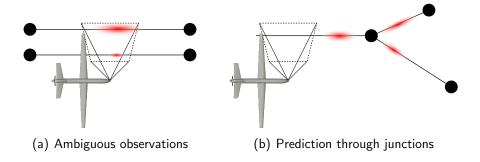
Figure 4.20: Examples of the two typical sources of multiple hypotheses in road-network-constrained parametric estimation.
