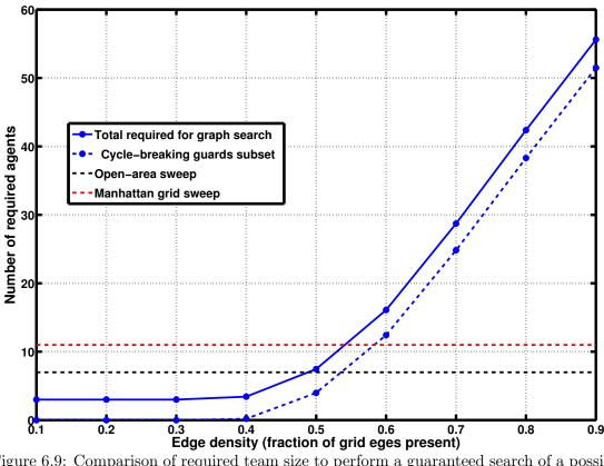
Figure 6.9: Comparison of required team size to perform a guaranteed search of a possibly cycle-containing road network of fixed  $3 \text{km} \times 2 \text{km}$  size and 200m edge lengths but varying edge density, from 10% to 90% of all edges in the underlying grid present. For reference, note that environments with these parameters and edge density 0.5 is considered canonically urban in this document.
