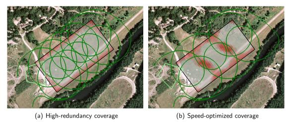
Figure 5.3: A comparison of two extremes in the resulting coverage pattern during a search, using (a) a high-redundancy (tight overlap) search and (b) a speed-optimized (low overlap) search providing possibly insufficient coverage of several interior regions. The level of coverage redundancy may be varied by changing a single parameter, the orbit-center precession rate. Colors and markings are as defined in Figure 5.2.
