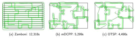
Figure 5.12: Sample execution results for three coverage algorithms in a suburban-density environment. Zamboni performs particularly poorly relative to the others because it is unvarying (up to random variation, exhibited here) in its path. Once again, OTSP shows better macroscopic optimality which is sufficient to outperform mDCPP, though some excessive maneuvering remains.
