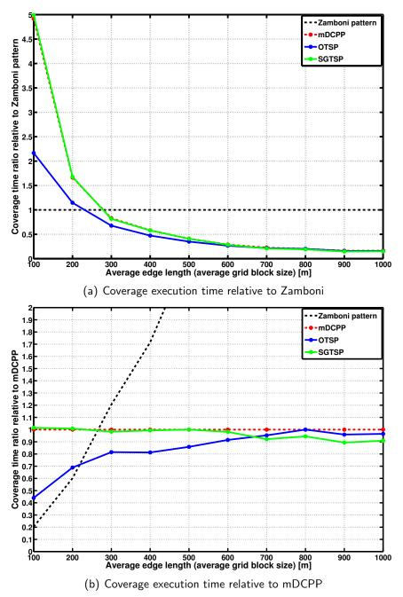
Figure 5.14: Coverage execution time comparison between a Zamboni pattern and the greedy mDCPP competitor, orbit TSP (OTSP), and sweeping generalized TSP (SGTSP) algorithms for a single vehicle. Note that for very dense environments, simple a Zamboni patterns is most appropriate. For less dense ones, OTSP is best. Finally, for very rural environments, SGTSP is preferable.
