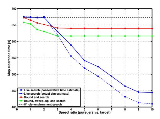
Figure 6.25: Comparison of mission duration with increasing searcher-to-target speed ratio to perform a guaranteed search for a bounded-speed target in a  $3 \text{km} \times 2 \text{km}$  road network with 40% edge density and block (edge) lengths of 700m (roughly, rural). The number of agents available to each strategy corresponds to the matching datapoint in Figure 6.22, that is, the minimum team size providing a capture solution is used in each instance.
