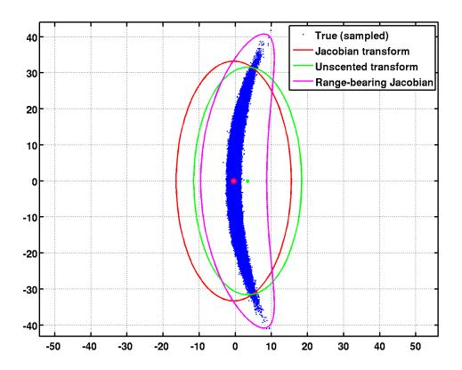
Figure 4.12: Comparison of uncertainty representation approximations compared with a monte-carlo sampling of the true distribution for a single observation with typical parameters (axis scale is meters), similar to Figure 4.8. Of these, a Gaussian uncertainty distribution represented in range-bearing space best matches the shape of the true distribution. The Unscented Transform in Cartesian space better captures the sample mean but remains constrained to a Gaussian.
