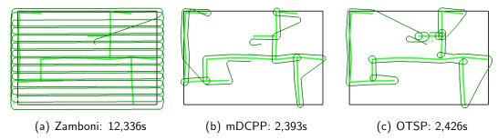
Figure 5.13: Sample execution results for three coverage algorithms in a rural-density environment. Here again, Zamboni performs particularly poorly relative to the others given the very small area of actual interest. Because it considers only full edges regardless of their length, mDCPP outperforms OTSP, which sequences more minute motions, though only by less than 2%.
