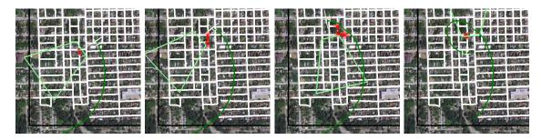
Figure 4.19: An example of pursuit in a road network using cellular decomposition. The UAV anticipates loss of view (area within the green trapezoid) and begins to turn sharply. While out of view, it predicts diffusion in possible target location (red probability mass) and greedily steers to maximize the probability of re-detection.
