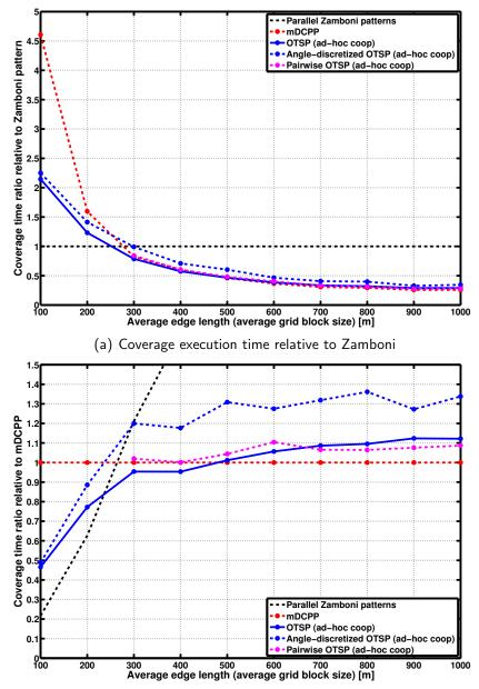
(b) Coverage execution time relative to mDCPP (note that pairwise is intractable in dense environments)
