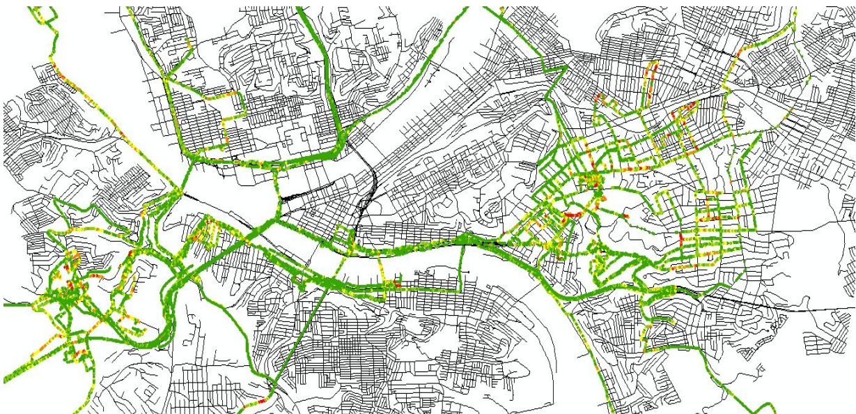
Figure 8 - Distress score overlaid on a GSI street map of Pittsburgh. Green, yellow, and red are low, medium, and high amount of cracks, respectively.
