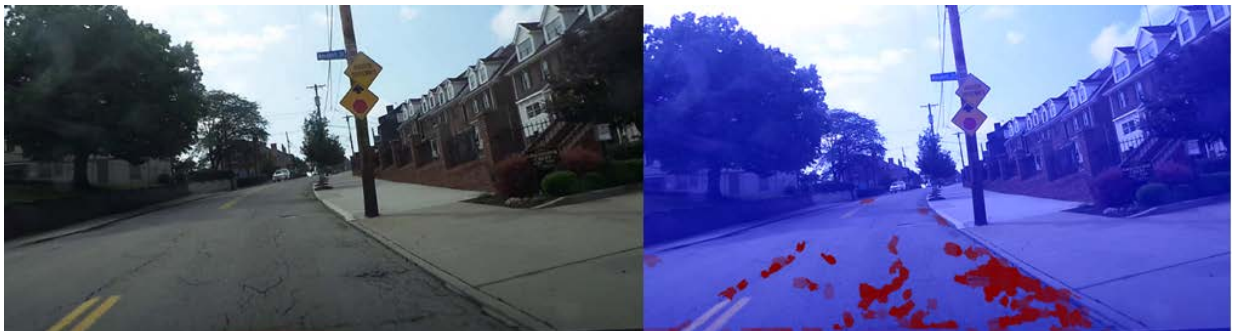
Figure 4 - Left: A typical road image with cracks in the road. Right: Classification result. The color indicates the severity of distress: blue = no cracks, light to dark red = light to severe cracks.
