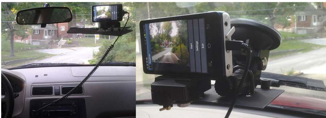
Figure 1 Data collection system: The smart camera is connected to a quick-release mount and fastened to the window with a suction cup. The camera is powered from the cigarette lighter. One can see the collection app running on the system.
