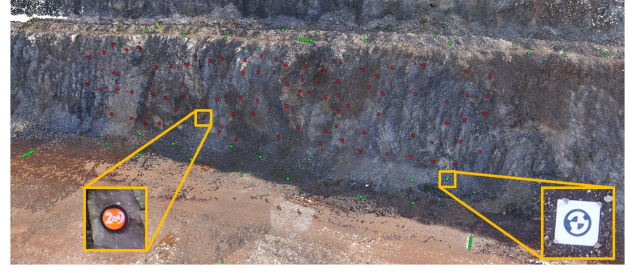
Figure 7: The reference point network allows an extensive accuracy evaluation. Systematic deformations of the image block and reconstructed object geometry can be quantified. Markers (bottom right) indicating GCP positions are shown in green, circular targets (left) for quantitative evaluation are in red.
