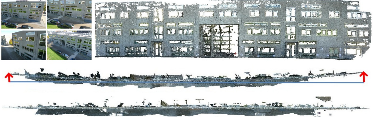
Figure 3: In the facade reconstruction using OpenCV calibration significant bending is prevalent (middle). In contrast, accurate camera parameters delivered by the method from (Daftry et al., 2013) results in a straight facade reconstruction (bottom).
