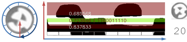
Figure 5: Histogram for an unrolled circular marker and rotation invariant binning of the code stripe. The numbers from top to bottom indicate the probabilities for center, binary code and outer circle. The marker with ID 20 has been successfully decoded.
