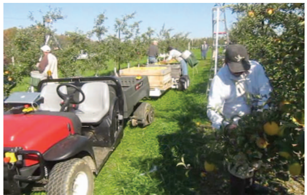
Figure 11. The autonomous orchard vehicle functions as a “bin dog” for workers harvesting apples. At the push of a button, the vehicle follows the workers as they pick the fruit and place it into the bins. When the bins are full, the vehicle takes them to the end of the row to be loaded into a truck. (Photo courtesy of Carnegie Mellon University.)
