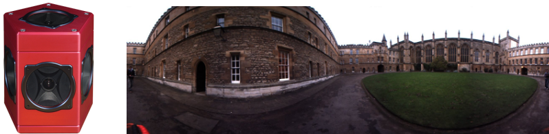
(b) Multiple camera array system (left) and stitched panoramic image (right).
