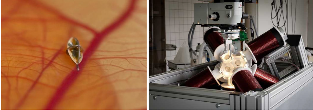
Fig. 2.11. Wireless magnetic microrobot for targeted retinal drug delivery. Photo credits [94], [96].
