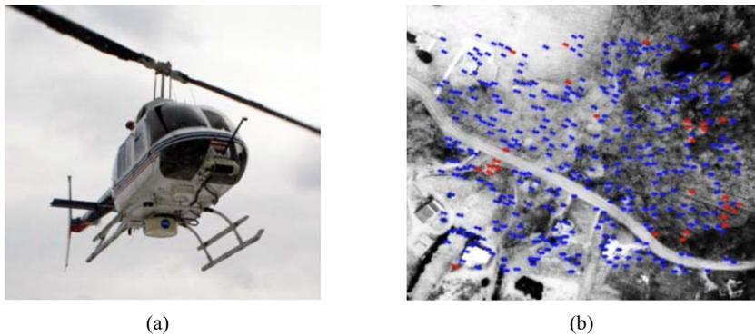
**Figure 6.** (a) Helicopter used in the experiments. A downward pointing camera is mounted to the front of the helicopter. (b) Tracked features. A total of 450 feature points are tracked between image frames. The red dots are outlier features assigned with zero weights in Algorithm 1. The blue dots are inlier features used in the motion estimation.
