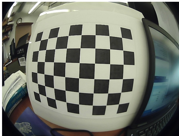
Figure 8 Example of the calibration target image from a fisheye camera.
