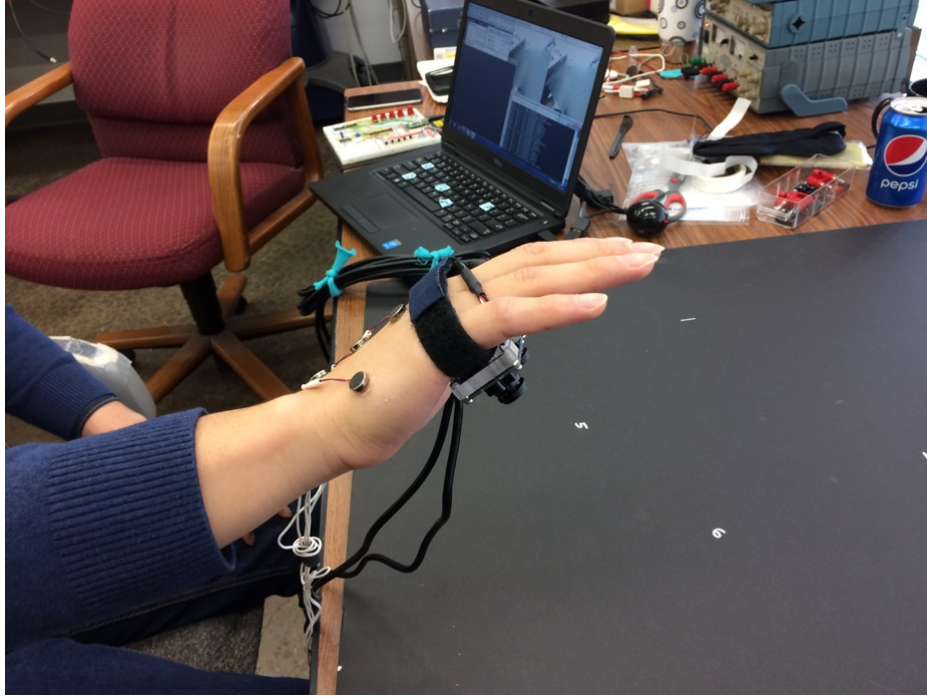
Figure 1 PalmSight apparatus, including stereo cameras, tactors, associated hardware interface, and laptop computer.
