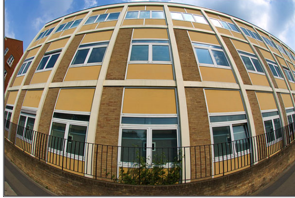
Figure 6 Image showing "fisheye" or "barrel" distortion.
