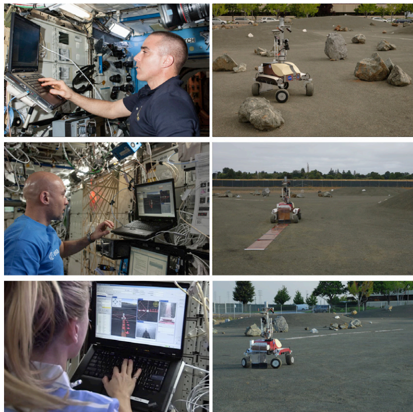
Figure 4. Surface Telerobotics testing. Top: site survey; middle: deployment of a simulated lunar telescope antenna; bottom: inspection of deployed simulated lunar telescope antenna.
