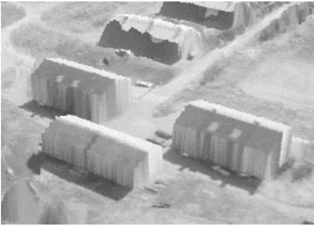
Figure 9: Three parametric peaked-roof surfaces that have been fit to DEM data within building boundaries hypothesized by Ascender. Compare with the raw DEM building data at the top of the image.
