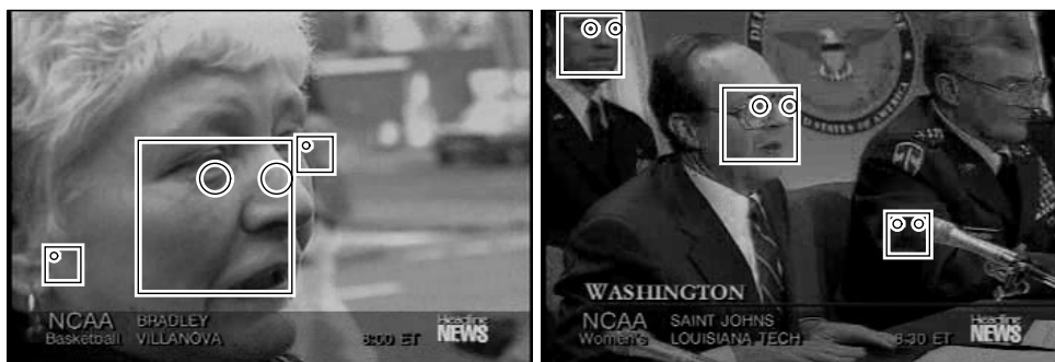
Figure 8: Detection of faces rotated out-of-plane.
