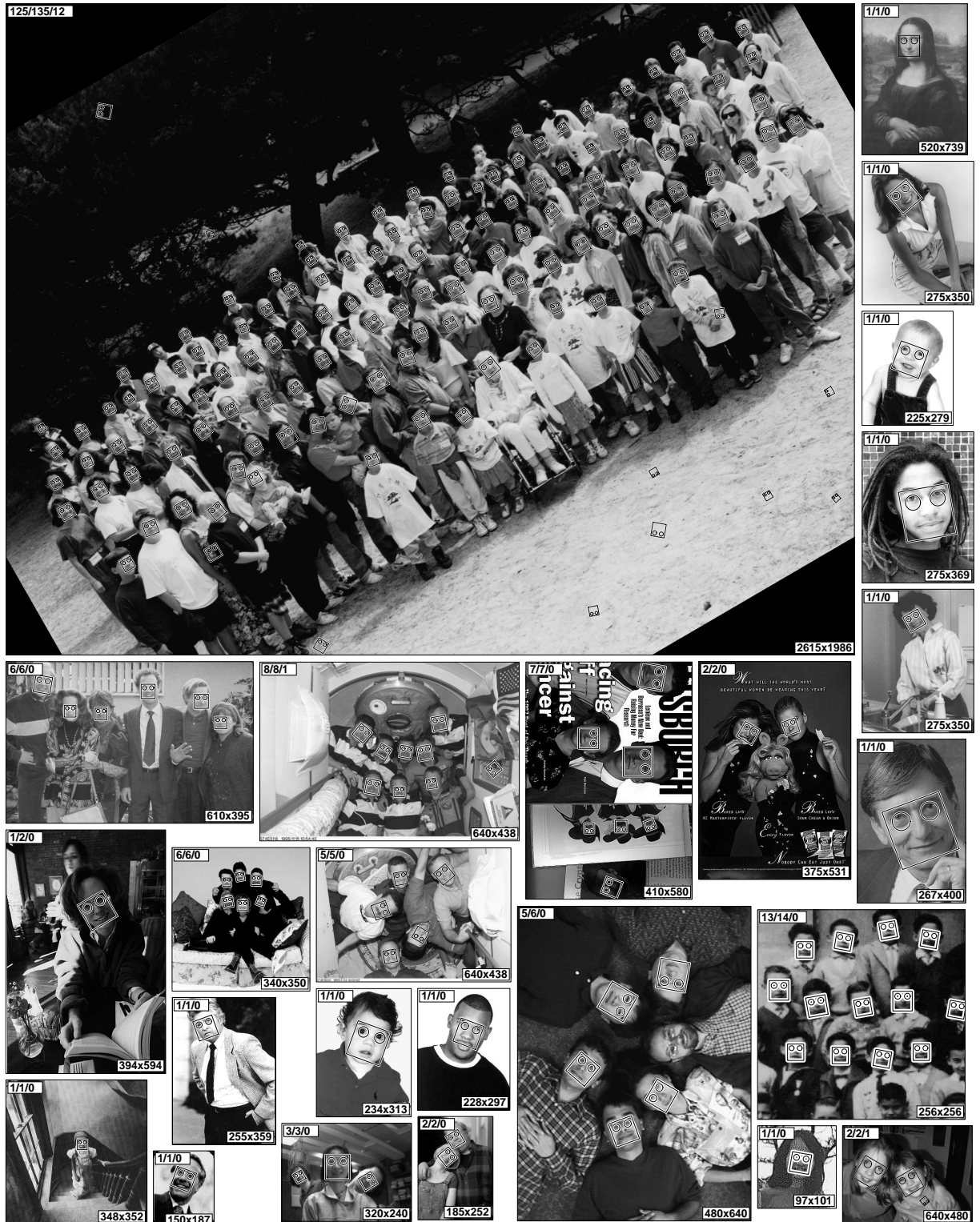
Figure 7: Result of arbitrating between two networks trained with derotated negative examples. The label in the upper left corner of each image (D/T/F) gives the number of faces detected (D), the total number of faces in the image (T), and the number of false detections (F). The label in the lower right corner of each image gives its size in pixels.
