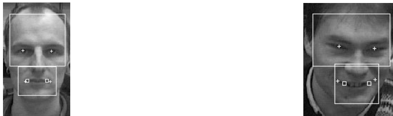
Figure 6. Initial search areas for the lips and found lip-corners. The small rectangles mark the predicted positions of the lip-corners.
