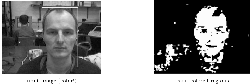
Figure 1. Application of the color model to a sample input image. The face is found in the input image (marked by a white rectangle)
