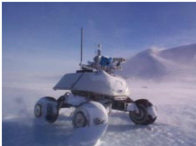
Figure 1: Nomad in the midst of a snowstorm in Antarctica. During its expedition to Patriot Hills, the robot endured wind chills as low as -70^{\circ}\text{C} and winds gusts up to 75 km/hr.
