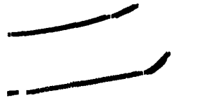
Figure 4. A classification of the laser reflectance scans in Figure 2, based on the absolute value of an edge operator. Black pixels indicate a potential obstacle.
