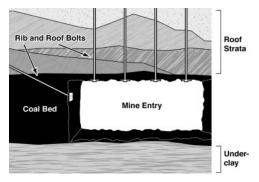
Figure 1. Underground Coal Mine Cross-Section
