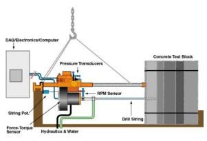
Figure 3. Laboratory Drill Apparatus and Setup
