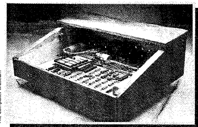
1976 Steve Jobs and Steve Wozniak design and build the Apple I, which consists mostly of a circuit board.
