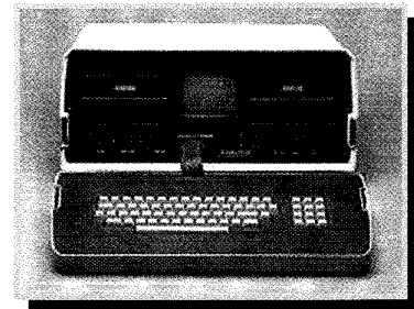
1980 The Osborne 1 “portable” computer weighs 24 pounds and is the size of a small suitcase.
