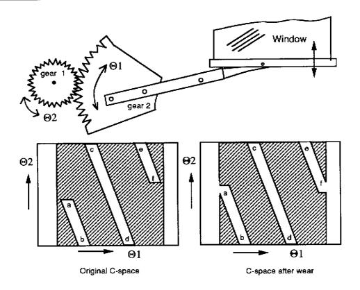
Figure 4-2: Example 2: Window Regulator Mechanism
