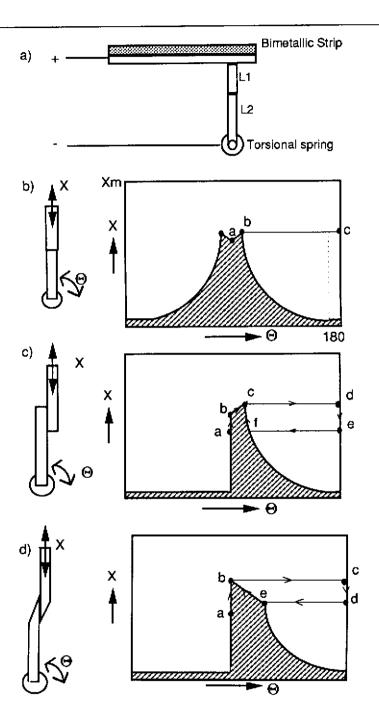
Figure 4-1: Example 1: Circuit Breaker
