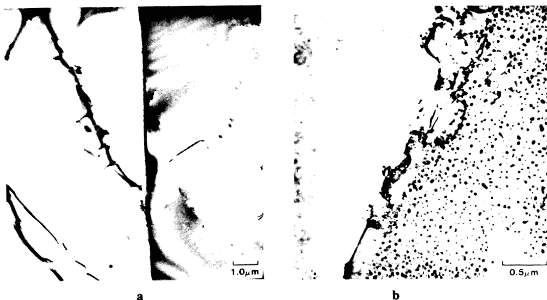
Figure 16: Micrograph of Al-3Li-0.5Mn; a. as Quenched, b. Peak Aged Condition (from [12])
