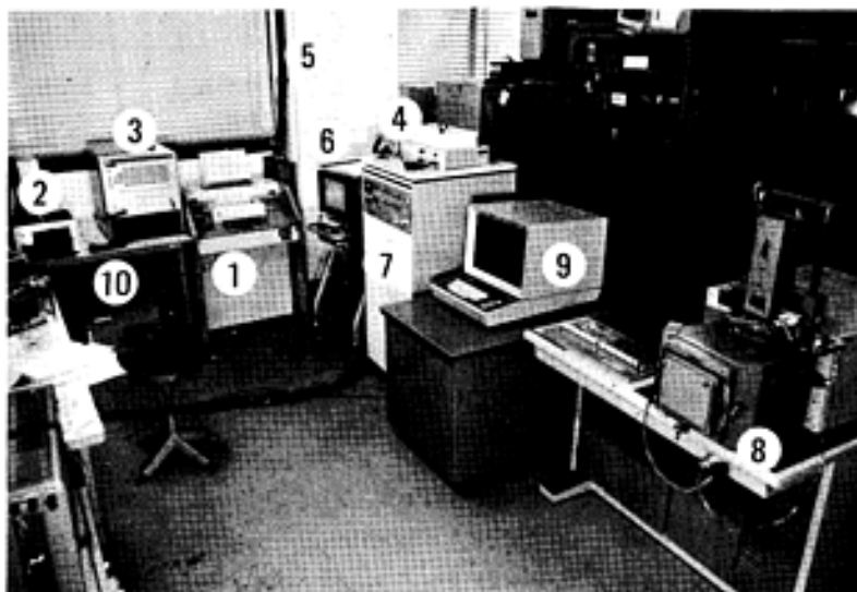
Figure 2-3 View of GIRLS subsystem: (1) I/O typewriter; (2) Paper tape reader; (3) CPU of MACC 7/F mini-computer; (4) Graf/pen; (5) Transmission cable to NEAC 2200/200; (6) Storage-type CRT; (7) GIRLS-interface controller; (8) Flying-spot scanner; (9) Character CRT; (10) Mini-disk device
